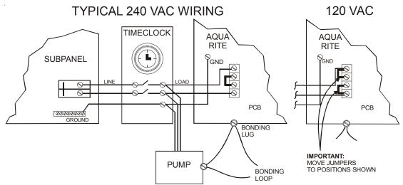
Note: Wire the pump directly to the timeclock--do not use the Aqua Rite as a junction box.
