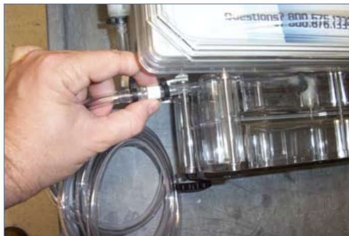
Figure 15 - Acid Injection line
