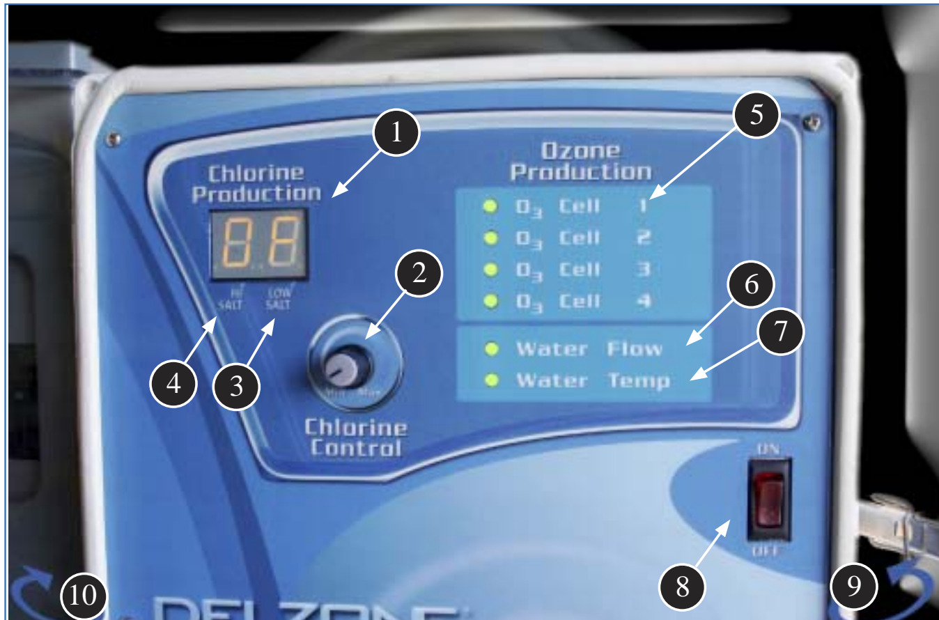
Figure 15 1. Chlorine Production Display 6. Water Flow Indicator 2. Chlorine Control Knob 7. Water Temp. Indicator 3. Low Salt Indicator 8. On/Off Switch 4. High Salt Indicator 9. Fuse (right side) 5. Ozone Production Indicators 10. Serial Number # (left side)
